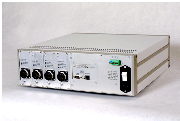
Primatics MDC-1400 Rack Mount Controller (RearView)
