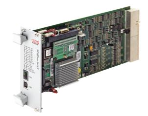
The SPiiPlusNT (NT - Network Controller) is designed for incorporation in the MC4U. Once plugged into an MC4U, the MC4U becomes also an EtherCAT master designated MC4Unt. It manages the EtherCAT network with up to 32 axes of motion and countless number of I/Os and sensor modules. The SPiiPlusNT also includes Servo Processors for controlling local drives that reside within the same MC4Unt enclosure.
